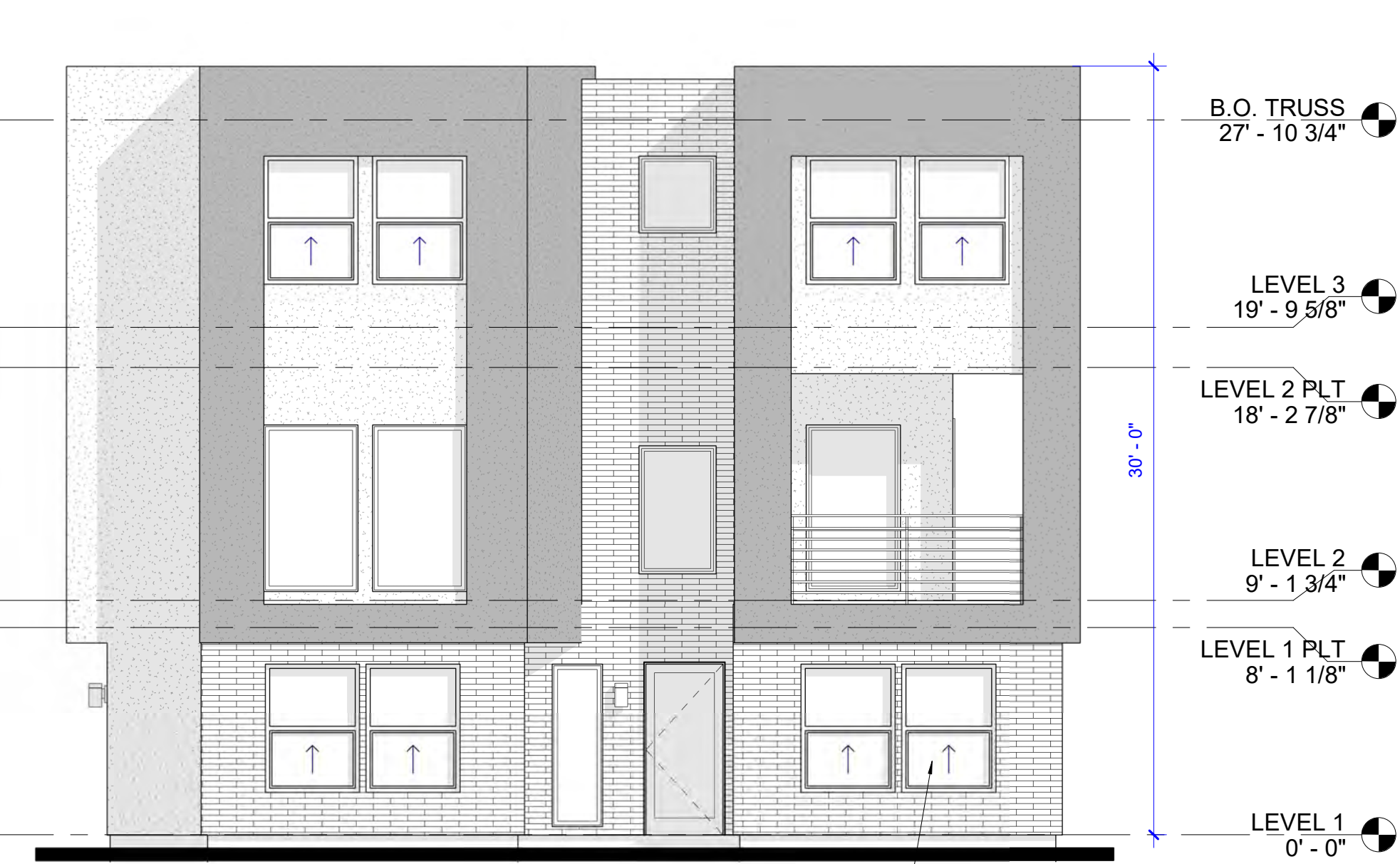
D1 BLD 1 WEST FACADE (STREET FACADE) 3/16" = 1'-0" TOTAL LEVEL 1 STREET FACING SQUARE FOTAGE: 302 LEVEL 1 STREET FACING GLAZING SQUARE FOTAGE: 86 (28.4 %)
